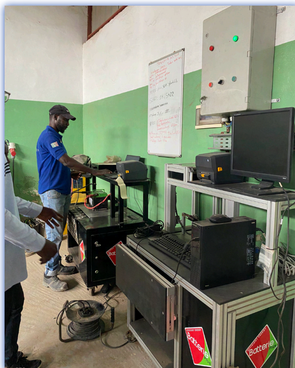
Figure 16b: Image of a workstation at BeEnergy equipped with digital monitoring tools, used for the controlled regeneration of batteries to ensure safety and quality.
