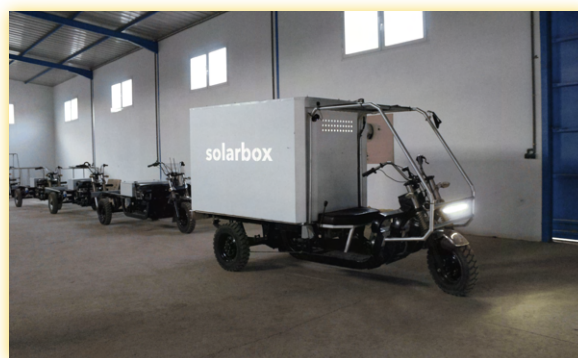
Figure 12b: Retrieved from the Launch Africa website. A Solarbox three-wheeler electric vehicle with a large cargo box, representing their locally built option for transport and delivery in Africa.
